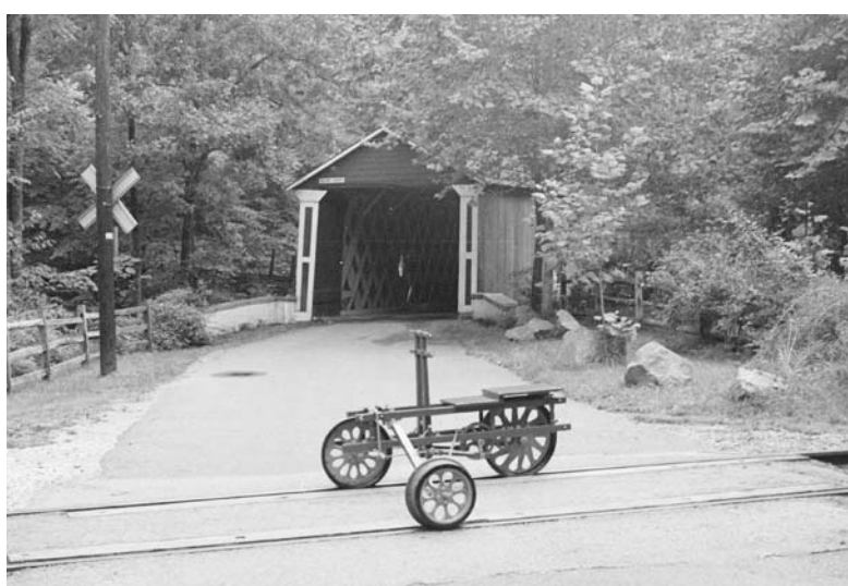
The editor's Sheffield No. 1 Velocipede at Wooddale in September 1992. After the Wilmington & Western Rail Road Company started using the line in 1872, velocipedes would have seen use after 1877 by workers for inspections and maintenance activities. A one-person velocipede was designed to carry a maximum load of 300 pounds. The No. 1 featured machine-cut gearing, ball bearing axles, and concave tread on the two large wheels to “practically eliminate the tendency to leave a wet or frosty rail”. Operating a velocipede is similar to sculling were the rider pushes pedals with their feet while pulling the vertical handle with their hands. The two handle positions serve as a “transmission”. The upper handles allow maximum leverage to get moving and then the operator uses the lower handles to keep moving and thus limit the rocking necessary for their upper body. Robert. E. Wilhelm, Jr. photo.
