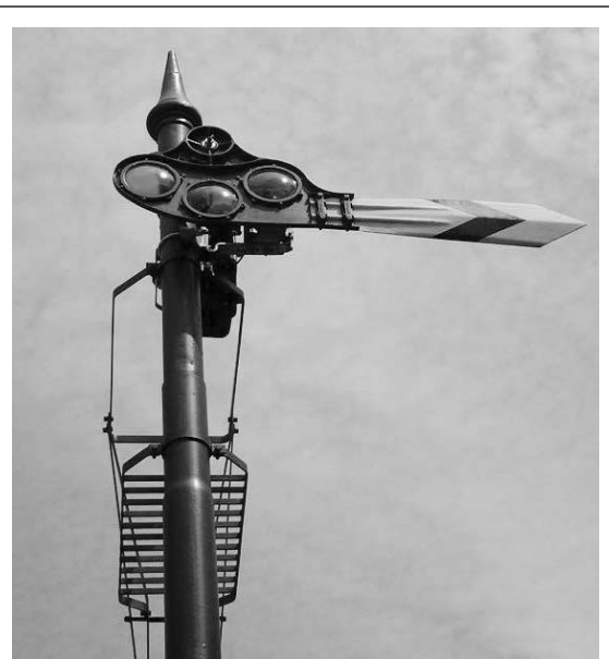
Greenbank Stations' semaphore signal is typical of over 25,000 units installed on American railroads. Dating from 1917 to 1919 the Greenbank example operated into the 1980s before being removed. August 30, 2015, Cristian Sanchez photo.
