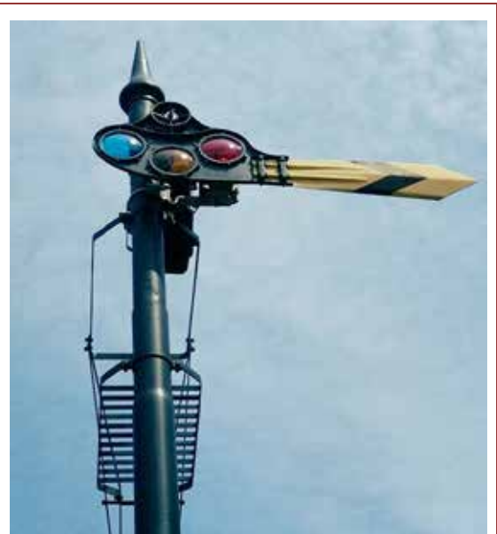
Greenbank Stations' semaphore signal is typical of over 25,000 units installed on American railroads. Dating from 1917 to 1919 the Greenbank example operated into the 1980s before being removed. August 30, 2015, Cristian Sanchez photo.
